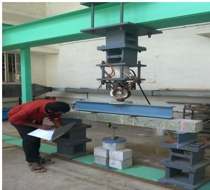
Fig.3: Loading Frame (Flexural Strength)
